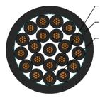
Annealed Copper Conductor LSZH Outer Sheath XLPE Insulation
